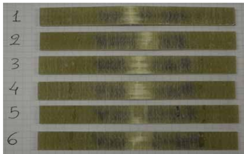
Figure 4 - GFRP with vinyl ester matrix.
