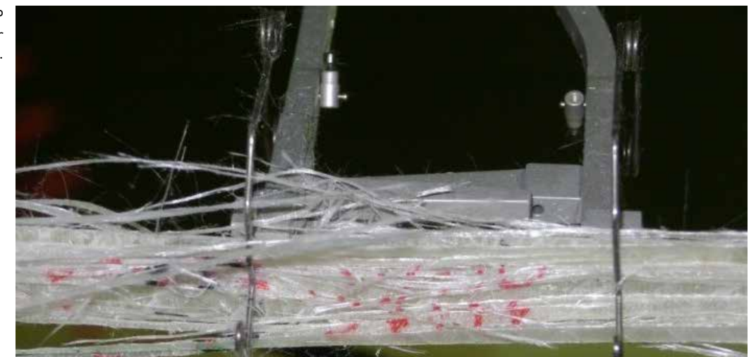
Figure 3 - GFRP with Sika® Biresin® CR83 epoxy matrix.
