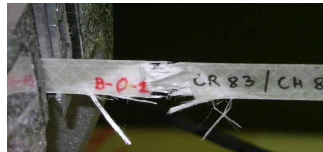
Figure 3 - GFRP with Sika® Biresin® CR83 epoxy matrix.
